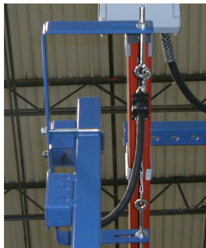
Proper alignment of Aeromotive energy rail and trolley
