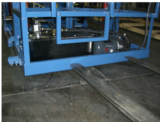
INCORRECT Pushing Extractor
